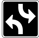
Two-way left turn lane
