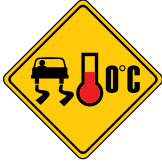
Surface subject to icing Bridge or roadway surface may be slippery at zero degrees Celsius — slow down
