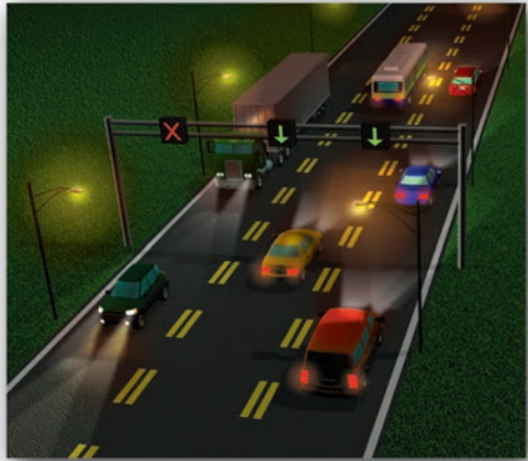
Lane Control Signal Lights
