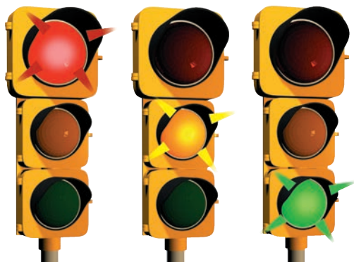
Flashing Red, Yellow, and Green Signal Lights
