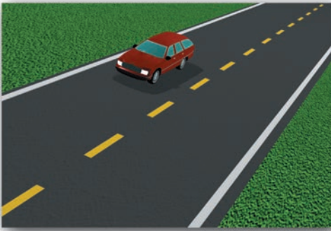
Broken Centre Line
