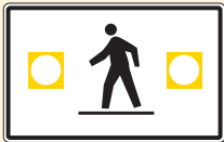
Pedestrian crossing signs with yellow lights.
